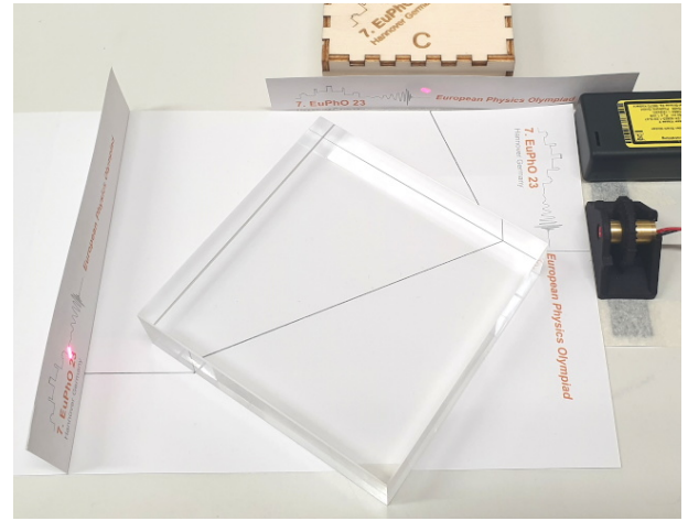
Figure 16: Determination of the laser polarization using Brewster reflection. The reflected beam will vanish at horizontal polarization.
